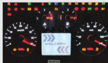
CAN Based Meter Cluster with Multi-Info Display & Gear Coaching feature
